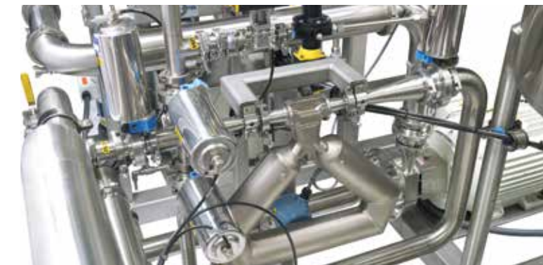
Precise Mass Meter-based blending ensures consistent product quality.
