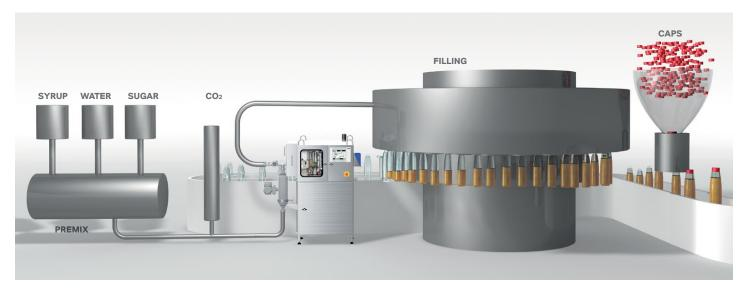
The Velcorin® dosing pump is installed in new or existing filling lines. Only minor modifications to the filling line are required for this purpose.
